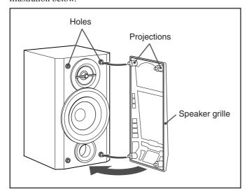
To remove the speaker grille, inserting your fingers at the top of the speaker grille, pull it towards you. Then pull the bottom towards you.
